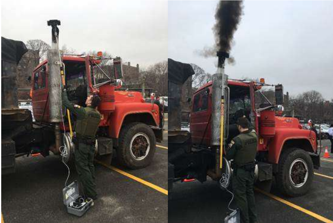
ECO Leubner operating emissions testing equipment on a vehicle in violation of air quality standards
